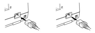
☐ Plug the other end of the power cord into a grounded wall outlet.
